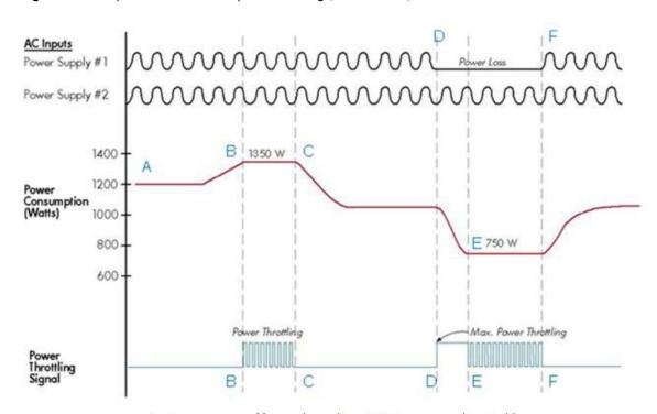
Figure 15. Example of AC redundancy with throttling (default mode)
